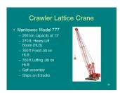
Construction managers will have to ensure that appropriate crane type and of required capacity is selected and utilized. Besides selection, placement, working radius as well as scheduling of crane has to be planned. Steel construction utilizes cranes for lifting heavy structural members. Crane rentals are very expensive so planning, scheduling and appropriate size selection are very critical. AISC has developed a detailed PowerPoint for learning crane selection, crane
