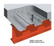
Composite construction with W-shape steel beams, composite deck and shear studs is very common in the US for floor construction of buildings. Composite construction reduces beam sizes and the construction costs. AISC provides a detailed PowerPoint presentation **Composite Construction** at <a href="http://www.aisc.org/content.aspx?id=21476">http://www.aisc.org/content.aspx?id=21476</a>
