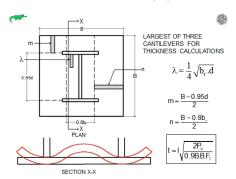
Construction students should learn about the design detailing structural properties and detailing of column base plates in detail. In the US tis part of steel columns creates many problems especially about the mis-alignment of the anchor bolts. The PowerPoints (i) **Shop Drawings** and (ii) **Column Base Plates** both provide adequate information about the base plates. Both PowerPoints are available in the conference folder at *ajayshanker.com*
