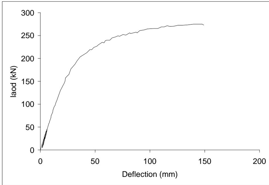
**Figure 4: Plot Of Load Versus Mid-Span Deflection For CB**
