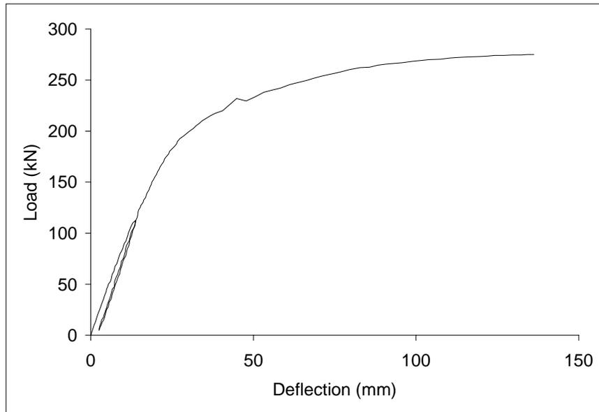
**Figure 5: Plot Of Load Versus Mid-Span Deflection For SB1**
