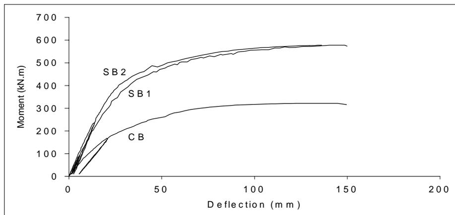
**Figure 3: Plot of moment versus mid-span deflection for CB, SB1 and SB2**
