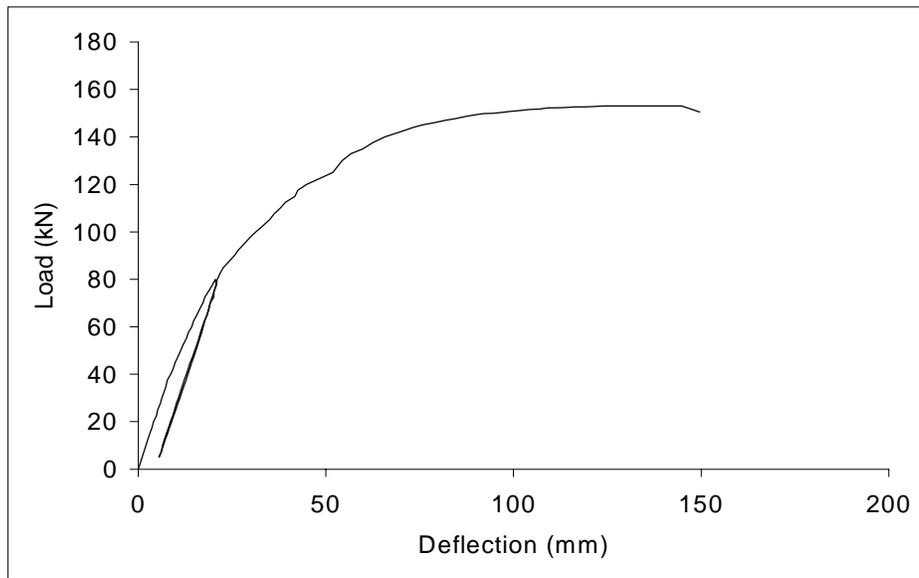
**Figure 6: Plot Of Load Versus Mid-Span Deflection For SB2**
