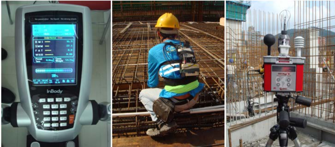
Figure 1: Various apparatus used in the field study (From left to right: InBody 230, COSMED K4b2, QUESTemp°36 heat stress monitor)
